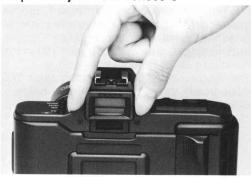
Ten eyesight correction lenses are available in powers of +3, +2, +1.5, +1, +0.5 0, -0.5, -2, -3 and -4 diopters. They may make viewing and focusing easier if you are near or farsighted. Slide the Eyecup T up to remove it before you attach the dioptric adjustment lens to the camera. Choose the one which is closest to your eyeglass prescription, and make a practical test if possible.
